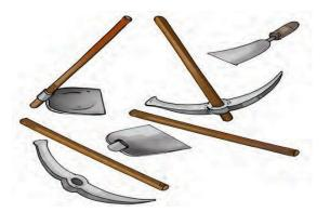
The iron blade of these tools has a ring in which the wooden handle is fixed. Normally, the ring is slightly smaller in size than the wooden handle. To fix the handle, the ring is heated and it becomes slightly larger in size (expands). Now, the handle easily fits into the ring. When the ring cools down it contracts and fits tightly on to the handle.
