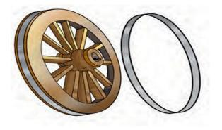
For fixing the metal rim on a wooden wheel of a cart. The metal rim is made slightly smaller than the wooden wheel. On heating, the rim expands and fits onto the wheel. Cold water is then poured over the rim, which contracts and fits tightly onto the wheel.
